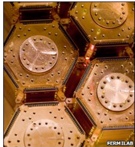
Detectors are designed to pick up heat deposits "left behind" by dark matter
