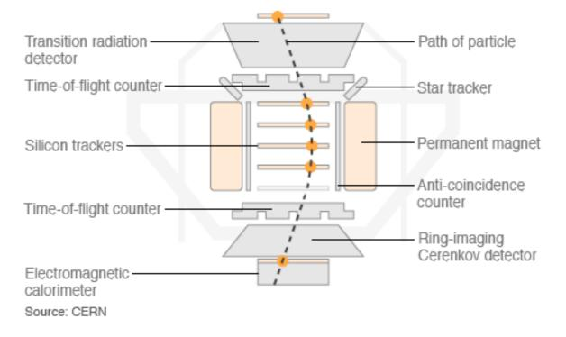
In the LHC, a ring of super-cooled magnets are used to accelerate and corral particles that have energies of 7 trillion electron volts (TeV). The cosmos-accelerated particles AMS will catch in its detectors may have energies of 100 million TeV. The Earth's atmosphere works to filter out such high-energy objects, so AMS has to go into space if it wants to study them directly.
