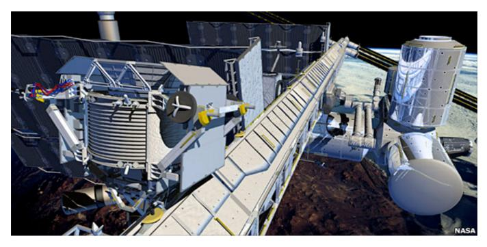
The AMS will sit on the station's truss, or backbone, slightly tilted to look past the giant solar wings
