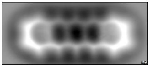
Even the bonds to the hydrogen atoms at the pentacene's periphery can be seen
