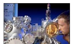
The measurement requires extremes of precision. In order to avoid the effects of stray gas molecules bounding around, or the general atomic-scale jiggling that room-temperature objects experience, the whole setup has to be kept under high vacuum and at blisteringly cold temperatures.
