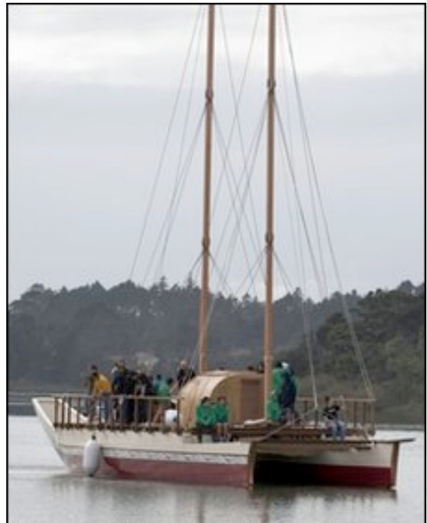
The boats are lashed together with wooden beams and ropes
