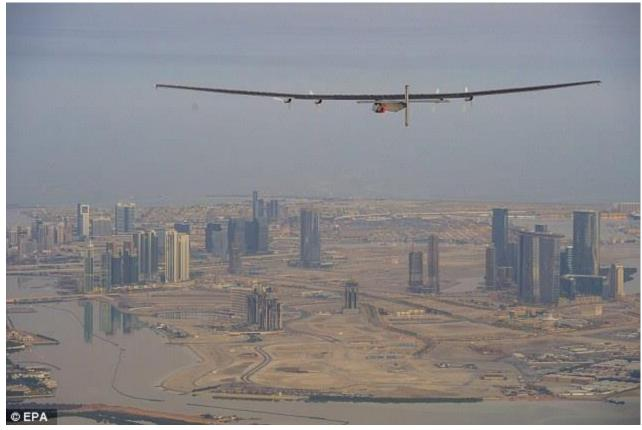
The 17,000 solar cells built into the wings supply four electric motors (17.5 CV each) with renewable energy. During the day, the solar cells recharge lithium batteries weighing 2,077lbs (633 kg) which allow the aircraft (pictured) to fly at night and therefore to have virtually unlimited autonomy
